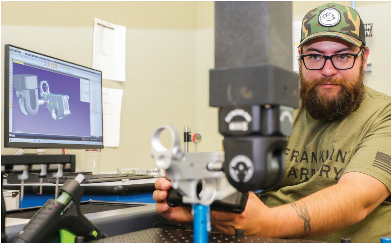
Above - Quality assurance manager Forrest is virtually self taught on the CMM thanks to the easy to use CMM Manager software that came standard on their Exact CMM. Right - The Renishaw PH-20 5 axis probe head was a must have on the CMM for its ability to access holes and slots deep inside a part.
